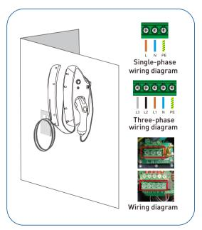
Note: The torque applied to the screws should be 1.8N-m to 2.2N-m  $\,$
